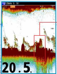
With the conventional color ranges, echoes from the seabed and a large fish are shown in a similar color, making it challenging to distinguish large fish from the bottom.
